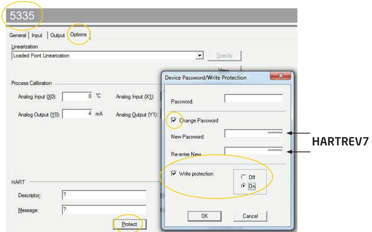
Switch **Write protection OFF** and write-enable the device by typing in the **Password "-CHANGE-"** in the top menu - acknowledge by pressing OK.
